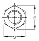
$\begin{array}{lll} d & = M20 \\ d \; max & = 21.60 \\ d \; min & = 20.0 \\ e & = 32.95 \\ m1 \; max = 10.0 \\ m1 \; min & = 9.10 \\ m2 & = 7.3 \end{array}$
